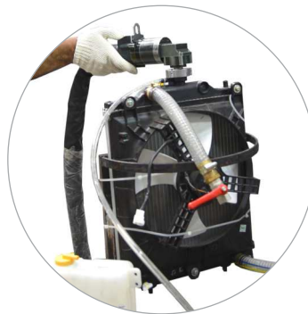
Radiator Coolant filling
